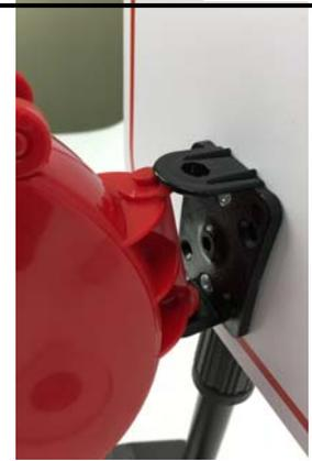
The Ticket Dispenser has two posts on the back of the unit that snap into the two holes in the mounting bracket. Line up the bottom post to the bottom hole and lift up/push back on the dispenser and it will snap into place.
