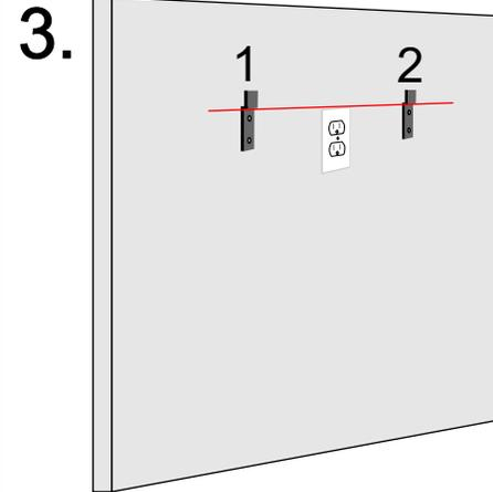
Make sure that the mounting brackets (red line) is above the electrical outlet.
